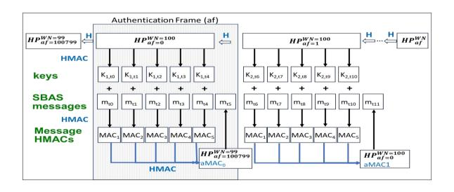
$$HP_{af_{i}}^{WN_{k}} = trun\left\{H\left(HP_{af_{i+1}}^{WN_{k}^{*}} \left\| \left.WN_{k}^{*} \right\| af_{i+1} \|S\right), 128 \; bits\right\}$$
